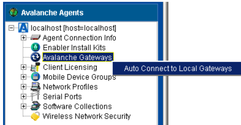
Figure 9-1. Connecting to a Local Gateway
